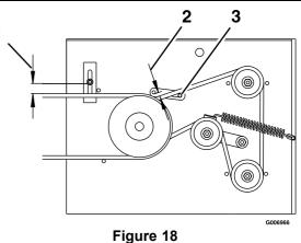
48 inch Belt Guide Location (Viewed from underneath the engine deck)
